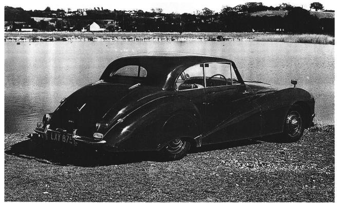
Early Tickfords had detail differences in appearance to the later ones. Where spats were fitted to the rear wings, then both front and rear wings had squared off lower corners. Later ones had radiused corners and no spats. Earlier cars had built in twin spot lamp while later cars had twin grills. C.l902 has dispensed with its semaphore arms and now carries Volkswagen rear and 'S' type Jaguar front turn indicators. As is well known, it is a much modified car.
